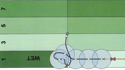
complete, then start back at shift #1. Repeat steps 1-4 until all shifts are Unhook the tow rope and leave the pod system to irrigate. Step 4:
