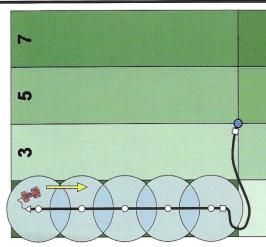
field and cross over the supply line. running, tow the pod line down the While the system is still Step 2:
