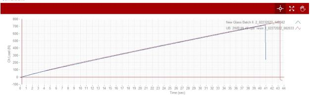
The 3 New Laminated Glass sample mean (average) was 513 Newtons. Safelite's Raz Hybrid Tool and HPX4 Resin 3 sample mean (average) after Thermal Cylcing was 398 Newtons.
