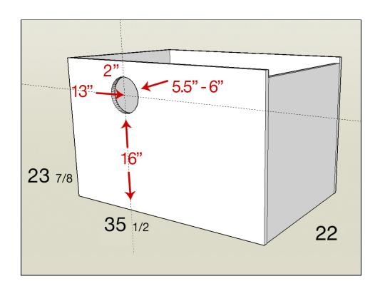
**NOTE: DO NOT GO OFF THIS IMAGE!** Entry hole/vent placement determined by site/wind. Most West Coast boxes will need hole placed on the right, not the left, because direction of wind will likely be out of the West.
