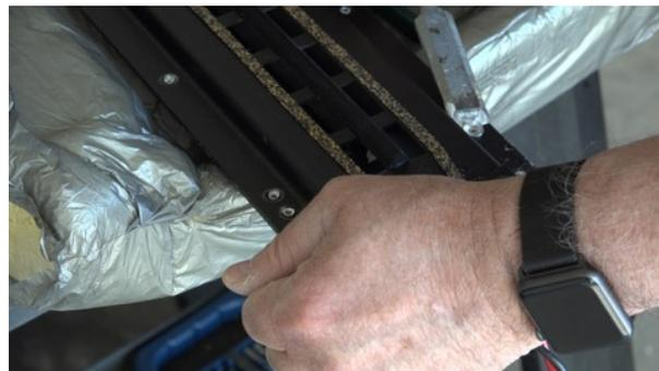
3. I had to clean the “puckey” from the contacts to get a better look at where I thought the break was. Failing that I started to pry the clamshell apart so I could get to the broken ribbon at the connecting circuit board that I had identified.
