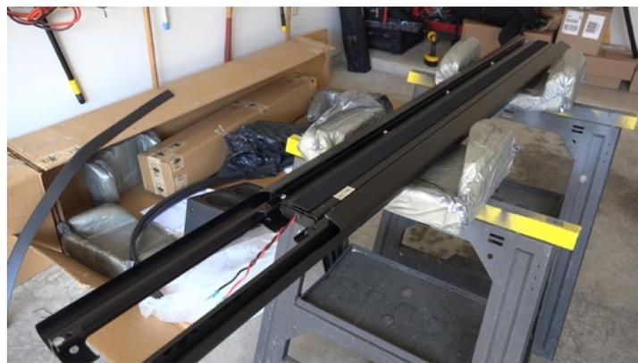
2. Once the ribbon module was completely removed from the frame I had to drill and remove all of the rivets that held the clamshell of the housing together.
