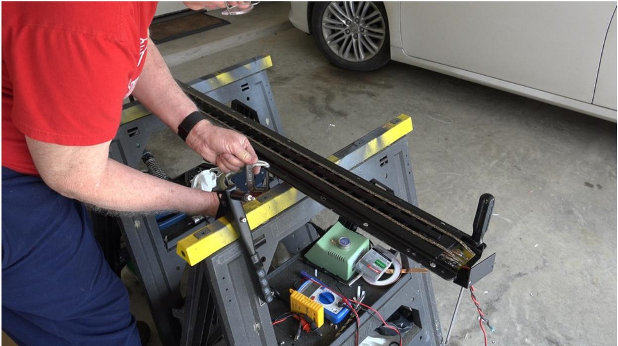
Moving the clamps as I placed the rivets assured that the clamshell was firmly and flatly riveted together.
