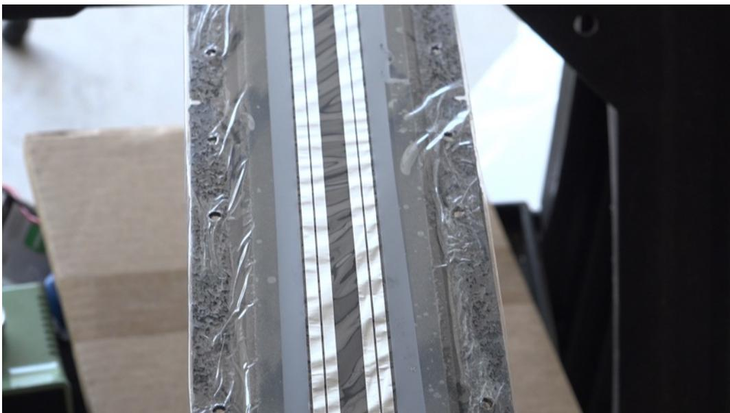
7. After trying to bridge the breaks in the connections with solder I discovered that the ribbons were too fragile to solder to effectively.
