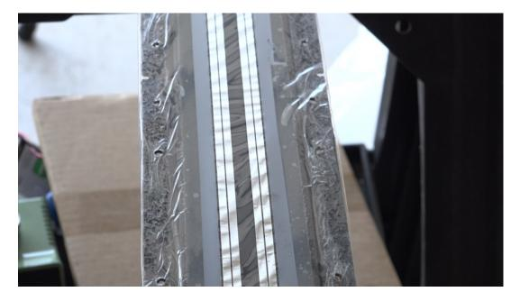
7. After tying to bridge the breaks in the connections with solder I discovered that the ribbons were too fragile to solder to effectively.
