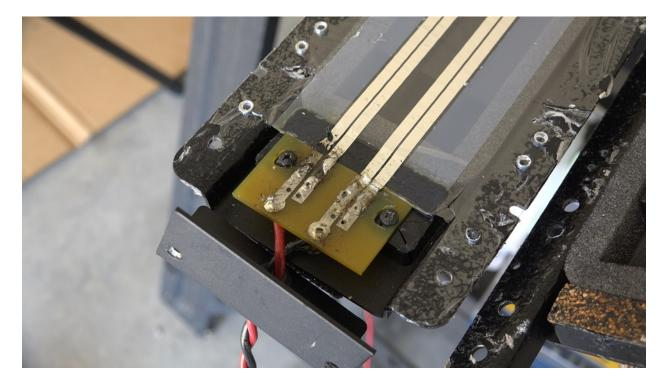
8. **New Plan Version 2.0** - I ordered some conductive foil with conductive glue to bridge the gaps but the glue would not adhere.
