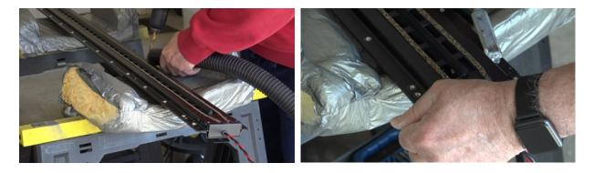
3. I had to clean the "puckey" from the contacts to get a better look at where I thought the break was. Failing that I started to pry the clamshell apart so I could get to the broken ribbon at the connecting circuit board that I had identified.
