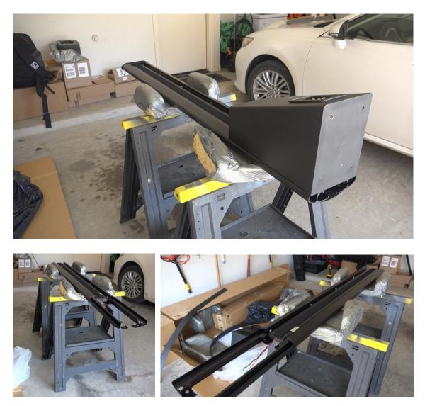
1. Dis-assemble the speaker to remove the ribbon module
