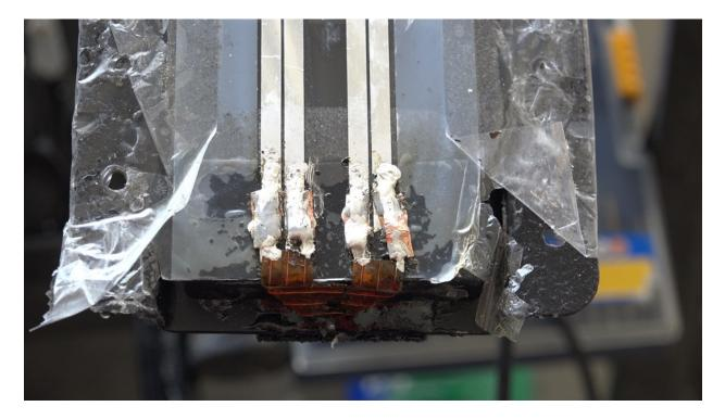
11. There were two retaining blocks (Squash Blocks) at each end of the ribbon that pushed down on the connections. These had a hard cork surface. Since I had built up the connections with the solder/conductive ink/copper foil I decided to replace the cork with some speaker gasketing material I had on had to provide a softer clinch while still restricting movement at the transitions from ribbon to connection block/PCB.
