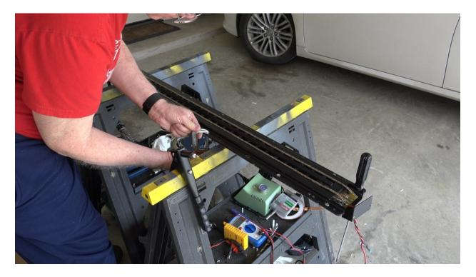
Moving the clamps as I placed the rivets assured that the clamshell was firmly and flatly riveted together.
