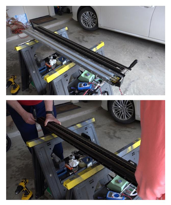
With some help from my wife we pressed the top and bottom halves together and I installed one rivet at each end to secure. This was not easily done since the powerful magnets in each half of the clamshell are set to repel the two halves! But, once the rivets were in I could install some clamps on either side to make sure the halves were firmly squeezed together before installing the rest of the rivets.
