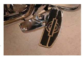
2. Using the **HEEL GUARD** as a template, place in rear corner of metal base plate. Be careful to align the rod with the inside edge of the base plate. Mark the holes first.
