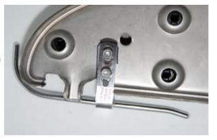
4. The finished Heelguard attached to the footboard (bottom of the footboard looking from front to rear).
