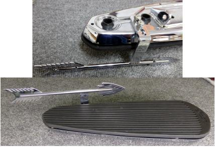
4) Re-assemble the footboard and rubber pad and re-attach assembly to bike.
