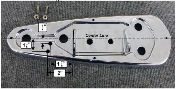
3) With the supplied 1/4" bolts arranged as shown below, attach the Heel Guard to the footboard and secure with the provide nuts and tighten the hardware using the supplied 5/32" hex wrench and a 7/16" wrench. You may use the slotted holes to adjust the location of the Heel Guard to your preference.
