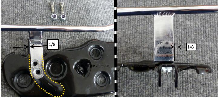
3) With the supplied 1/4" bolts arranged as shown below, attach the Heel Guard to the footboard and secure with the provide nuts and tighten the hardware using the supplied 5/32" hex wrench and a 7/16" wrench.
