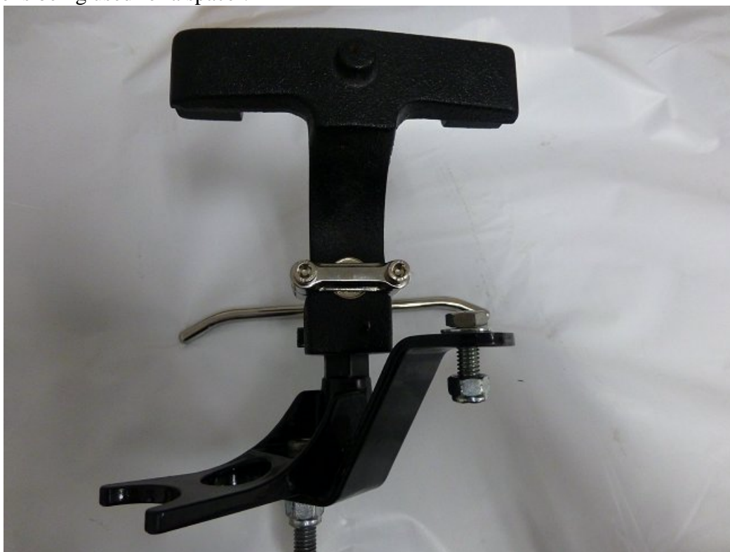
Photo #3 – Final Underside view with heel guard clamped to mounting bracket. Note the dime is being used for a spacer.
