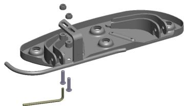
4) Tighten the hardware using the supplied 5/32" hex wrench and a 7/16" wrench. Top view shown below:
