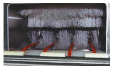
With all pre-cleaning equipment debris is removed from the side, upper and lower surfaces of the sack and this debris can be extracted and contained within an integral or existing plant dust extraction system.
