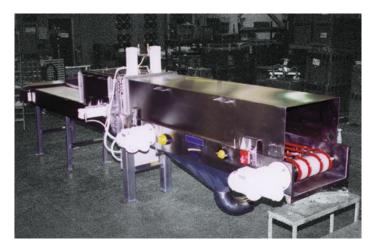
**Sack pre-cleaning systems** remove unwanted debris from the external surface of the packaging, prior to entering the next processing stage. There are 4 precleaners available in the range:
