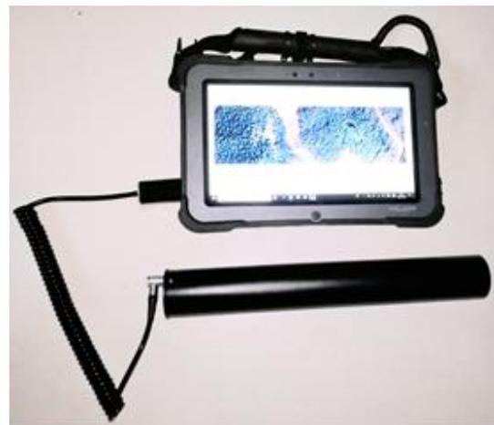
The CS30A probe and the rugged tablet connect directly as the walking detection system.
