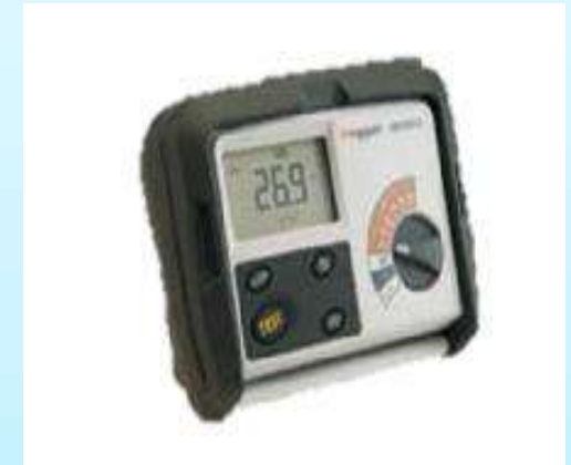
Earthing resistance test kit - Megger
