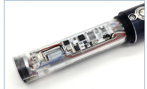
2) Carefully remove the battery. This is most easily done by lightly tapping the end of the chassis against your hand. Remember the chassis is marked to ensure, on reinserting the battery, that the positive and negative ends line up correctly.
