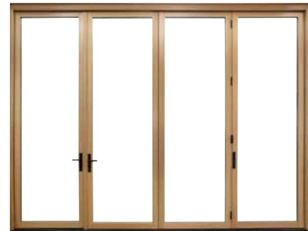
**Dramatic folding glass walls** with up to 8 panels can accommodate openings over 24' x 10'. | **Narrow 3 ¼" stiles** enhance and maximize the view. | **Hinged panels** fold accordion-style to the outside along a fixed track. | **Concealed shoot bolt** system releases the shoot bolts while providing a handle for ease of operation when opening the panels.
