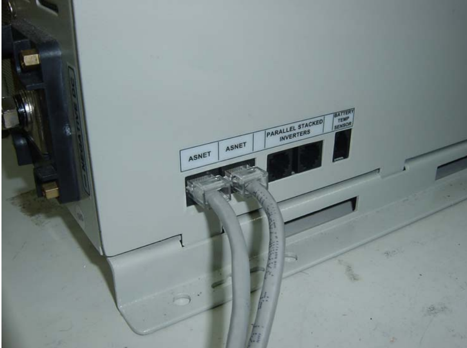
The first Inverter communication ASNET interface
