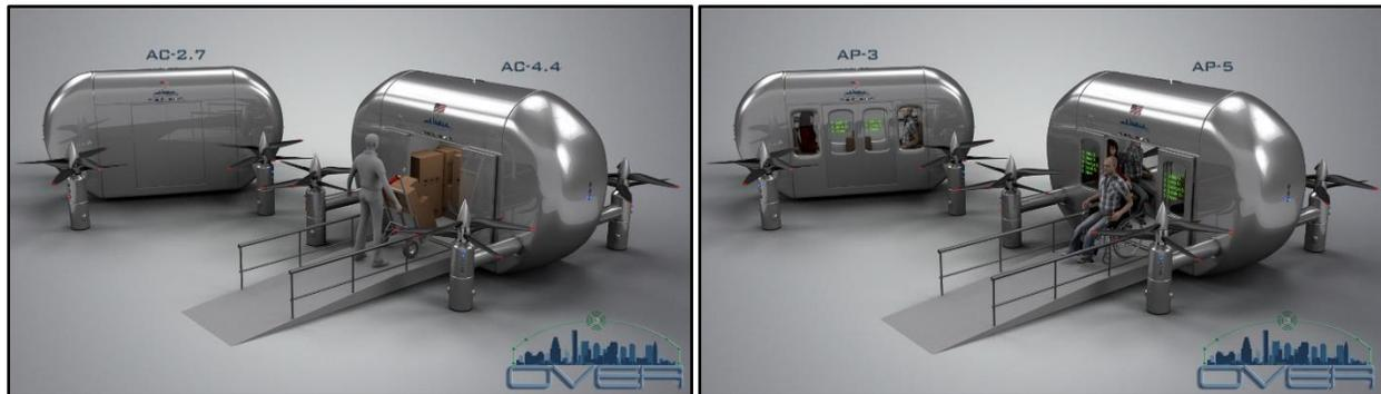
The illustrations show handrails on either side of the ramp, which is *incorrect*. Handrails would *not* be used on ramps due to close proximity to propeller blades. However, ramps will have “curbs” at least 2” high on either side (see illustrations below), to prevent people or cargo from rolling or falling off the side. The ramp provides safe, convenient access for customers with wheelchairs, strollers, walkers, luggage, and various rolling cargo devices and containers.
