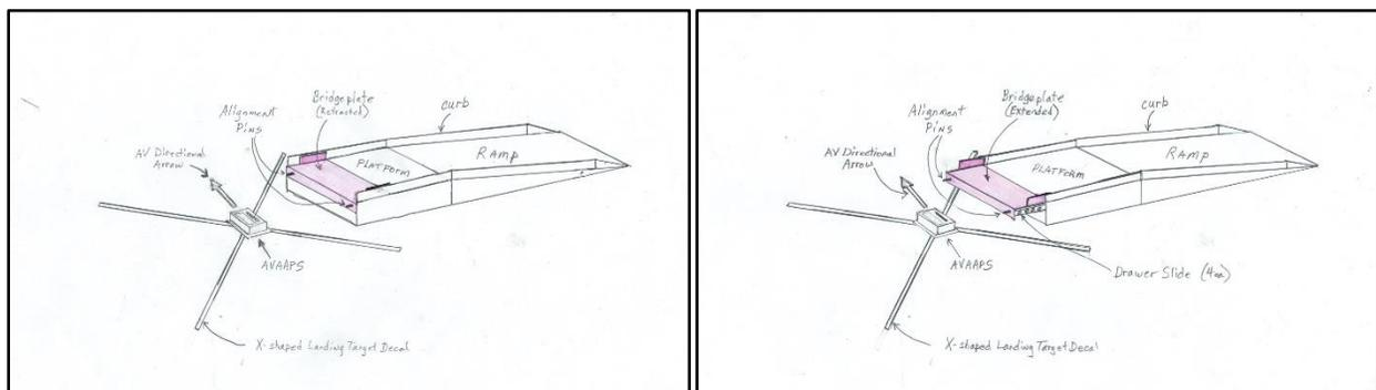
**Arrival Procedure:** When the Pad Assembly receives the wireless “ANCHOR” signal from the AV, its control circuitry sends a +12VDC signal via the STP cable to the RPBS’s actuator, to extend the bridgeplate. Once received, the +12VDC moves the actuator outward, to *extend* the bridgeplate until rubber bumpers contact the AV, at which time it stops. While extending, two alignment pins
