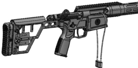
This firearm was originally sold with a key-operated locking device. Although it can help provide secure storage for your unloaded firearm, any locking device can fail. All firearms are designed to fire if they are loaded and the trigger is pressed. Therefore, never install the locking device inside the trigger guard or in any way that makes it possible to press the trigger! Do not leave the keys in the lock.
