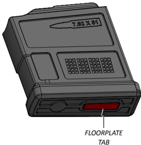
2. Slide the magazine base plate forward and remove the floorplate, spring and follower from the magazine tube.
