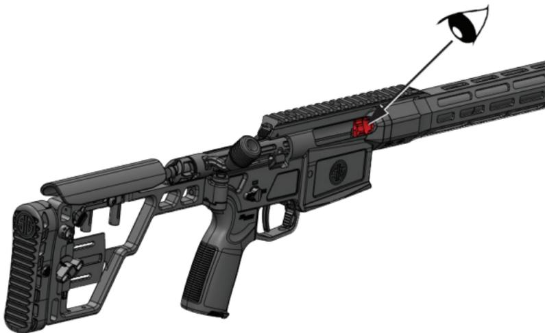
5. If you're passing the firearm to another person, allow that person to inspect the chamber prior to relinquishing the firearm. Pass the firearm with the bolt to the rear and the safety selector lever on SAFE.
