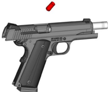
4. Unload and clear the pistol, as described in Section “5.0 Unloading and clearing the Pistol” on page 44. If you fire the pistol until magazine is empty, slide will remain locked to the rear. If you want to continue firing, reload pistol, as described in Section “3.5 Reloading During Shooting” on page 34.
