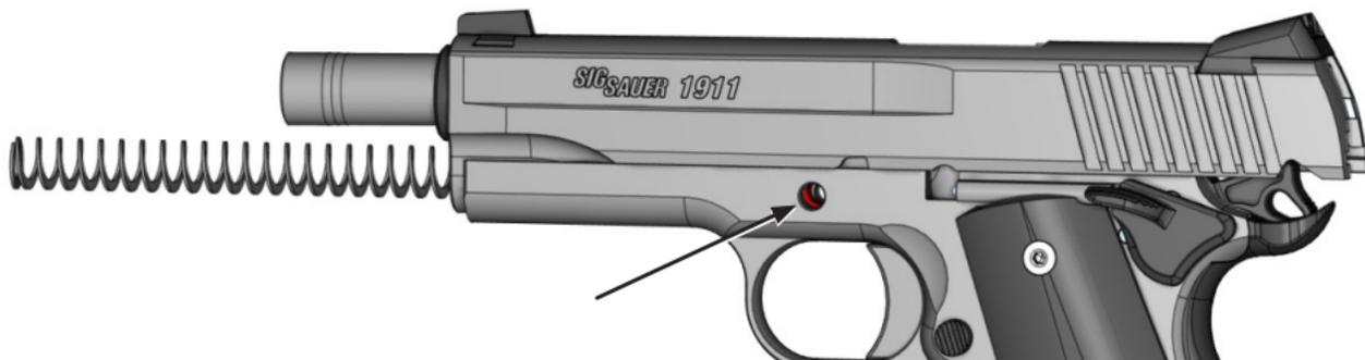
8. Insert slide stop shaft through frame so it passes through barrel link.
