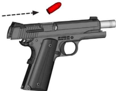
4. Visually and physically check the chamber, magazine well, and breech face to ensure that the pistol is completely free of ammunition.
