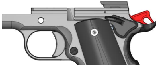
6. Align the rails on the frame with the slots on the slide and push the slide onto the frame.
