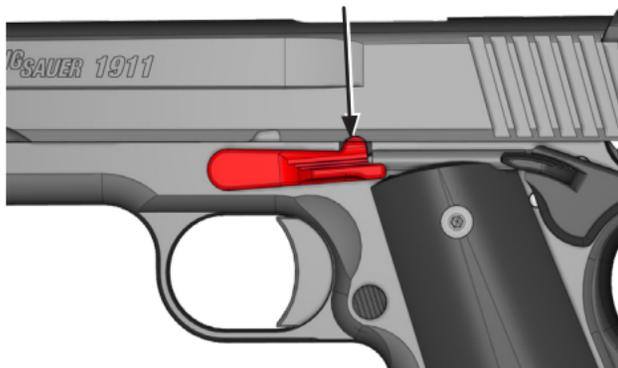
5. Push the slide stop lever out of the frame from right to left.
