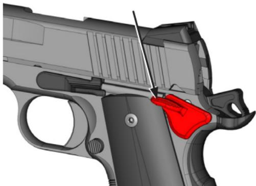
*THUMB SAFETY DISENGAGED (LEFT SIDE)*
