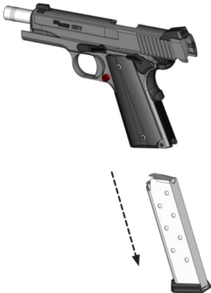
2. Insert a loaded magazine, pushing it up into grip until it locks in place. You should hear an audible click.
