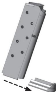
3. Slide the spring insert out to remove the magazine follower and magazine spring from the magazine tube.
