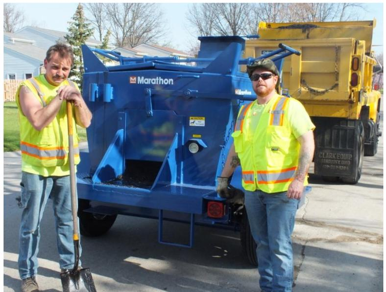
After several delayed delivery dates, Kevin and Red waste no time getting out to use the township’s new 2-ton Hot Mix Asphalt Hot Box Hauler. The equipment was purchased through the State of Ohio Cooperative Purchasing Program and will be used for patching pot holes and small asphalt repairs. This equipment will not only save time and money but will provide a better, longer lasting patch and allow the road crew to fill pot holes even during inclement weather.
