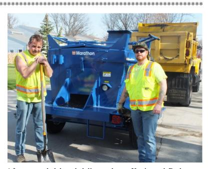
After several delayed delivery dates, Kevin and Red waste no time getting out to use the township's new 2-ton Hot Mix Asphalt Hot Box Hauler. The equipment was purchased through the State of Ohio Cooperative Purchasing Program and will be used for patching pot holes and small asphalt repairs. This equipment will not only save time and money but will provide a better, longer lasting patch and allow the road crew to fill pot holes even during inclement weather.
