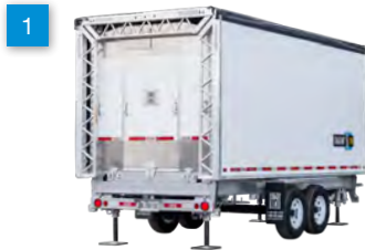
Trailer levelled with hydraulic stabilizers. Optional.
