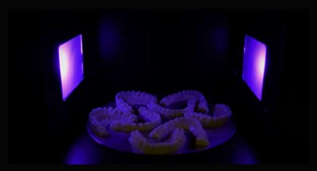
X3D Cure features a 360° turntable and a reflective base. Unlike some of the other UV chambers that use mercury lamps, X3D Cure uses duel UV led diodes power rated 20W. The light source produces no ozone, which is much more environment-friendly and energy-saving. The lamp life can last up to 10000 hours, ensuring you can cure your prints for a long time. Its UV led wavelength ranges 370-405nm.
