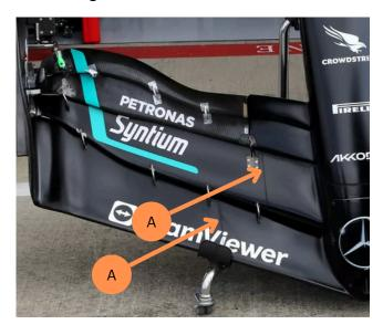
Excessive split lines can lead to increased weight and a poorer quality surface finish resulting reduction in aerodynamic load. It is important that the 60% scale WT model uses the same split lines at the FS components to ensure updates are compatible.
