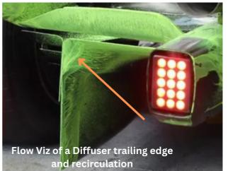
The photos of Flow Viz are then used to validate CFD & WT . By comparing the visual results with the numerical simulations, we can ensure that those models are accurately representing the physical flow phenomena.
