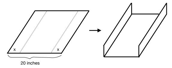
a. Express the cross-sectional area of the gutter, A, as a function of its depth, x.
