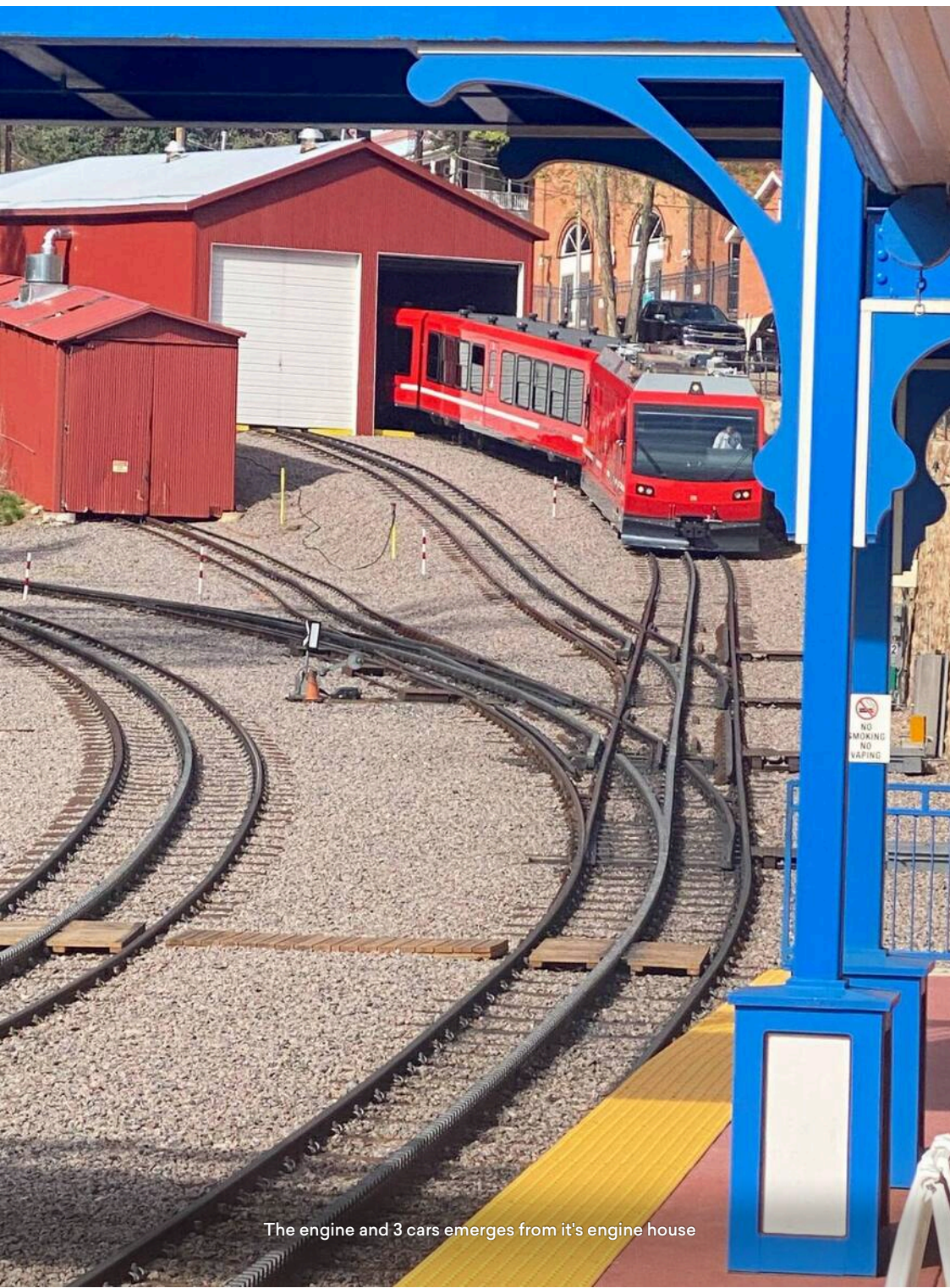
The engine pushes the cars up the hill with the engineer driving from the front car.
