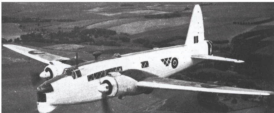
Vickers Wellington Mk XIV with Retractable Leigh Light
