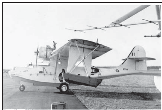
A Canso A (Amphibian) similar to that flown by 5 (BR) Sqn was the amphibious derivative of the Catalina flying boat.
