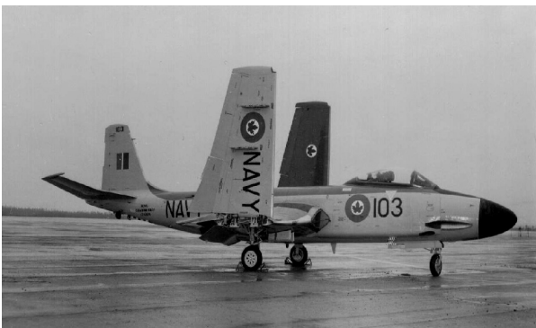
Photo caption: Royal Canadian Navy Banshee jet fighter with wings folded. DND photo.
