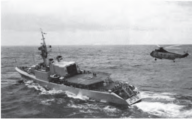
A VX 10 Sea King landing on HMCS Assiniboine during Beartrap test and evaluation trials.
