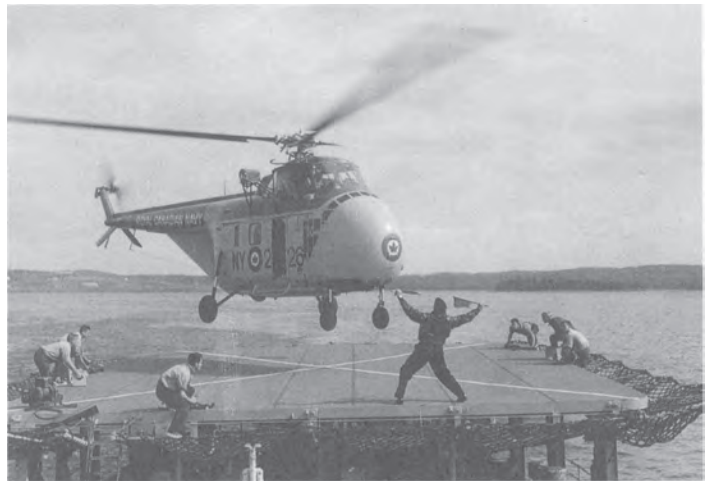
An HO4S helicopter landing on HMCS Buckingham. The makeshift flight deck was used to prove the concept of helicopters landing on small ships. Note sailors with chains at the ready to secure the HO4S to the deck.
