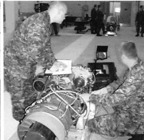
Technicians working on a Sea king GE T-58 engine versus maintenance demonstration on the Cyclone GE CT7-8A-1 Engine
