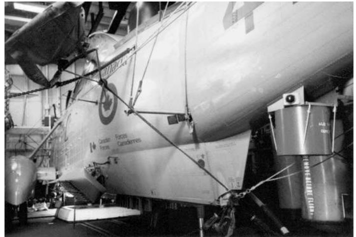
24 August 1990 ~ Day of Departure 413 in ATHABASKAN's Starboard Hangar Sporting the IR Jammer Protective Cover Designed and Fabricated by Shearwater
