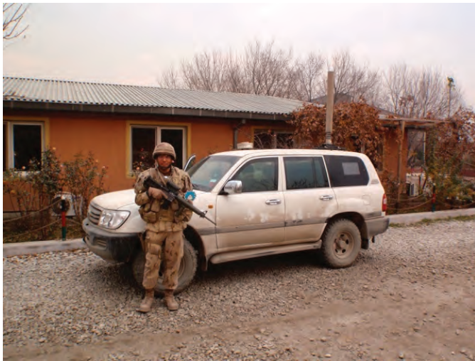
Loaded up for a trip outside the wire in our uparmoured Toyota Landcruiser. The antenna on the back is a cell phone jammer to prevent IED (Improvised Explosive Devices) that are triggered by cell phones.
