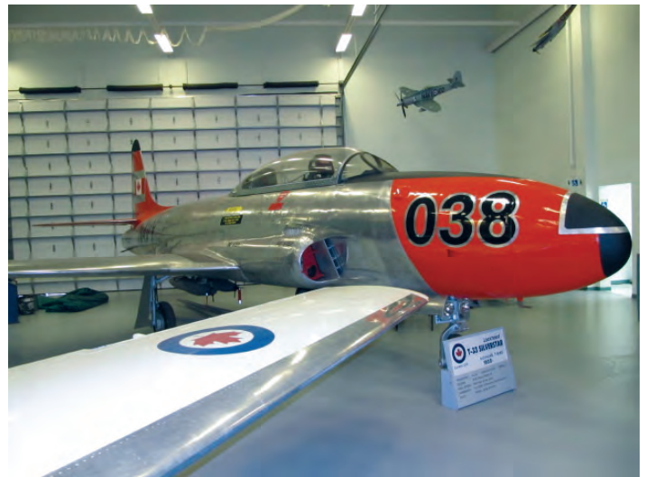
CT133038 Lockheed "Silver Star" (T-bird) after its restoration was completed. The T-Bird was used by the RCN at Shearwater in the 1950's and 1960's for pilot proficiency training and towing targets.
