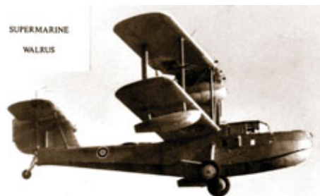
Walrus Z 1781 in RCN (FRU 743) service. Note the yagi radar antenna on the outboard forward wing strut. DND/PAC/PA-135609.
