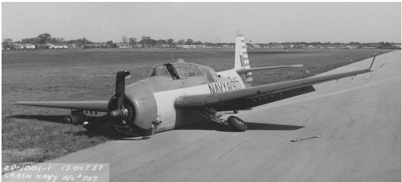
Here's what happens when your oleos have a bad case of arthritis. DND/RCN photo.
