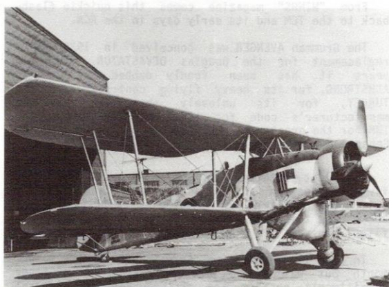
Shown above is an earlier Swordfish restoration, circa 1948. Note the exhaust collector ring similar to that contributed by IMP. Photo courtesy Guy Laramee.
