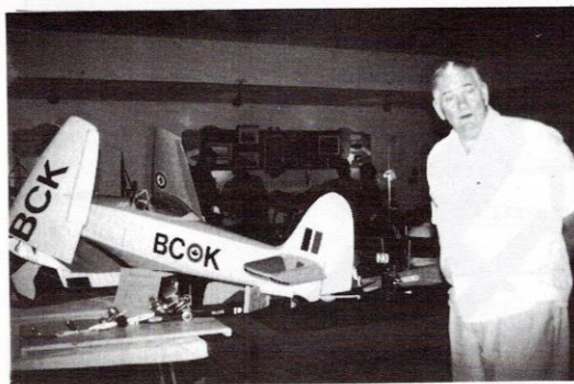
Former C2AT4 Ted Peters is shown next to the fully flyable Fury model he recently presented to the SAM. Made from fibreglass and balsa, and weighing 37 lbs, it is powered by a 4.2 cu in Sachs engine.
