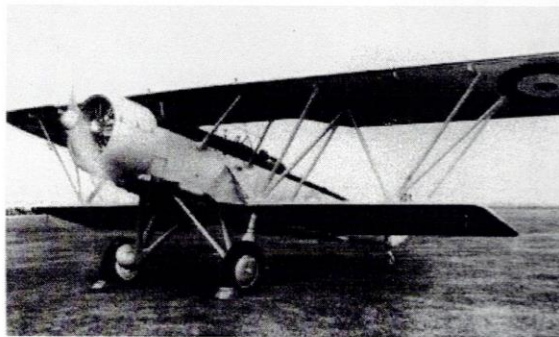
RCAF Shark on wheels as used on HMS Puncher rather than its more usual float configuration)
