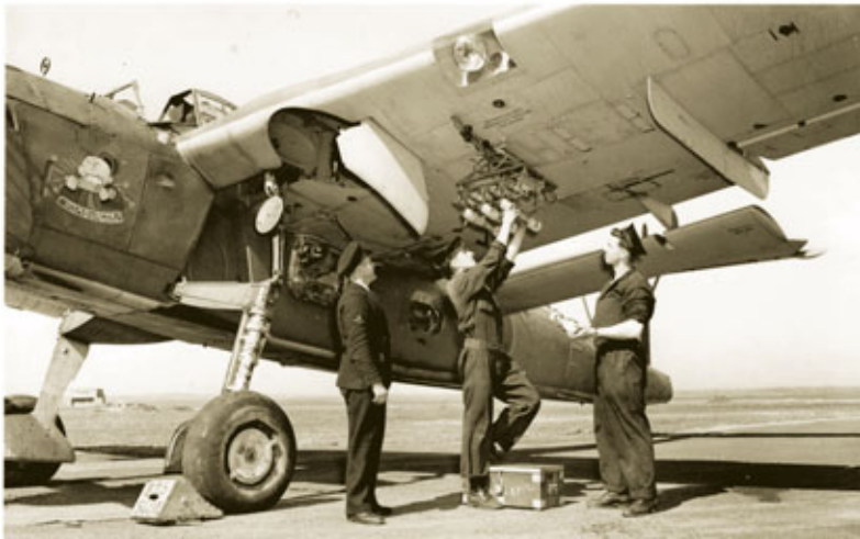
Personnel of 825 Squadron, RNAS Rattray, Scotland, August 1945: AM/O Orel Murdock affixes a 12-pound smoke bomb to a light-series bomb carrier on a Barracuda II, AM/O Elmer Rutledge stands by with the fourth bomb, and PO Allan McKenzie looks on. DND photo.
