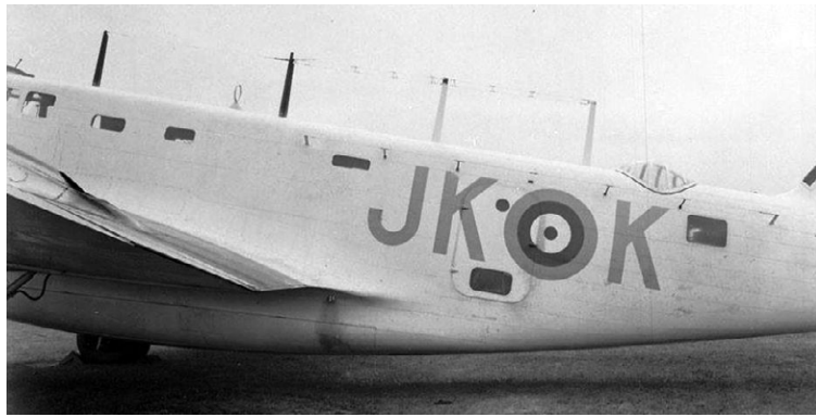
ASV II Radar Transmit Antennae On Top of Fuselage Dipole Receive Antennae Along Upper Side of Fuselage
