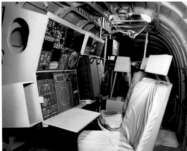
Figure 2: A period mock-up of the new Side Facing Console for installation of the APS-503. The radar can be seen in the middle, with the ASN-501 in front of the TACCO on the left. The mock-up still includes the AQS-10 sonar, which was changed to the AQS-503 before the fleet modification was performed. Photo from the Shearwater Aviation Museum archives.
