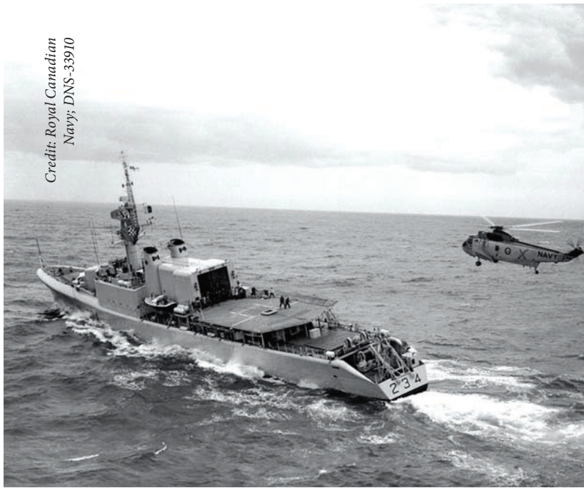
The Helicopter Hauldown and Rapid Securing Device, or Beartrap, was introduced on the RCN's destroyers, enabling Sea Kings to operate from small decks in almost any condition. Here, a Sea King approaches HMCS Assiniboine some time before September 1964. The rectangular Beartrap can be seen on the deck.
