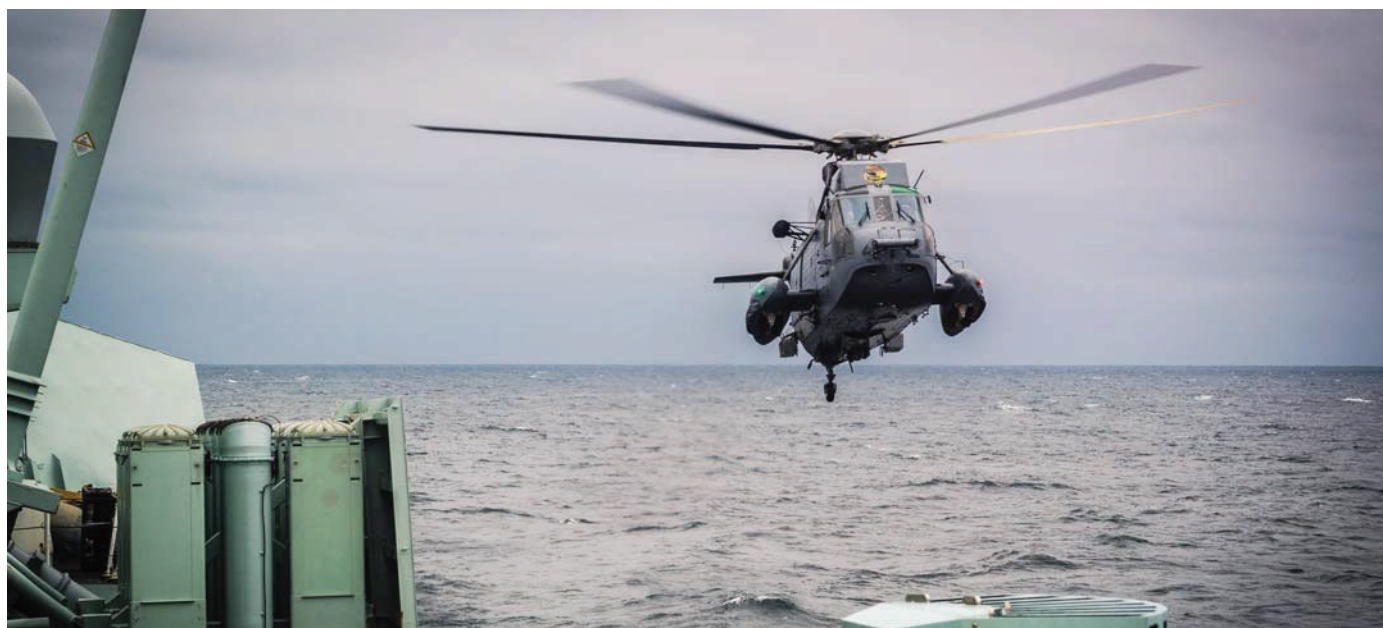
A Sea King helicopter, nicknamed Blackhorse, flies next to HMCS St. John's during Operation Reassurance in the Baltic Sea in March 2018. This view shows off the helicopter's boat-like 'keel' and somewhat awkward sponsons.
