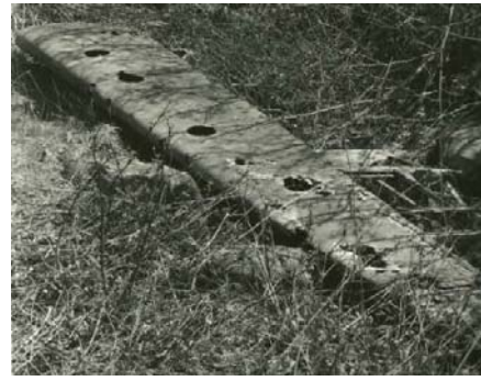
Left : Retrieving a manikin from X 4555 at the McNabs Island training site. Right : The forward section of an X 4555 wing. Both photos show machine-gun ports -- but no evidence of cannon -- in the wing leading edges. These are diagnostic traits of the Spitfire. Both photos via Lee Walsh.
