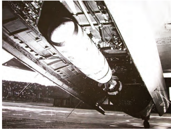
Mark 43 homing torpedo installed in an RCN Avenger bomb bay.
