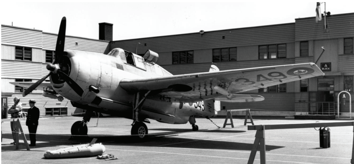
NAVY * 349 on exhibit at HMCS Naden at Esquimalt BC. Note the depth charges loaded on the undersides of both wings.
