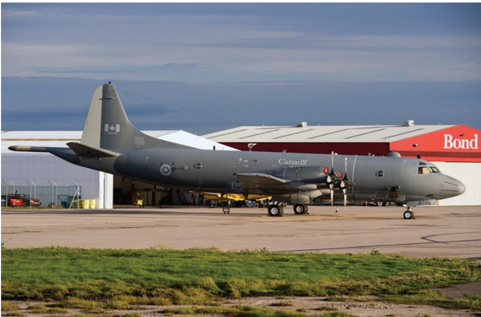
A BLOCK III AURORA with the dome just ft of the cockpit housing the BLOS antenna
