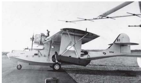
Yagi Radar Antennae Mounted On Wing (Foreground) And Fuselage
