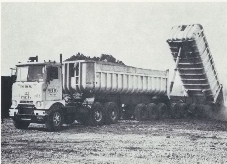
At left, one of the new 42 cubic yard GMC tandem rear axle tractor rigs is dumping clay. Each tractor pulls a triple-axle dump semi-trailer and a five axle dump full trailer. These light-weight, high-strength diesel trucks form the base of a new firm led by veteran industrialist Roy Fruehauf. The tractors were designed and constructed for the construction industry and adapted for hauling peak payloads under Michigan's axle weight laws. This fleet of trucks is considered by veteran construction men to be breakthrough in the field of tandem earth moving.
