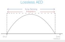
Lossless AED sensing: 1 step required Simultaneous X-ray sensing & Charge integration
