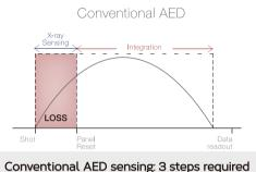
1. X-ray sensing 2. Panel reset 3. Charge integration
